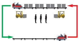
**Equipment Requirement:** 1 - Tugger 4 - Trailers (4,000 Lbs. Capacity) Quad-Steer 2 - Forklifts (4,000 Lbs. Capacity)
